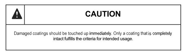
If these rules are observed, your product can be stored for a longer period. Please remember that elastomer parts and coatings become brittle naturally. If the product is to be stored for longer than 6 months, we recommend checking these parts to ensure that they function correctly. If replacement is necessary, please consult the manufacturer.
